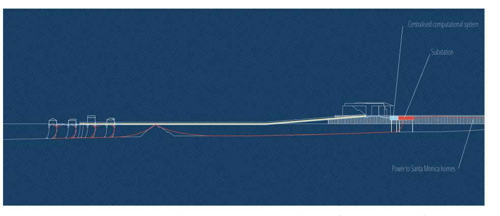
A centralised computational system, integrated within the existing pier structure, calculates the amount of energy produced by the flotation buoys and initiates the production of fog when the energy production increases at beyond the specific targets. Water is drawn from the ocean into a centralised pumping system and pumped along pipes under the floating walkway. Once the pipes reach the grid, they are connected to each of the 128 follies.
