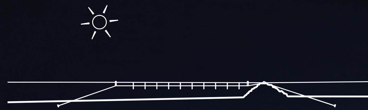
Wave power system section - normal weather
