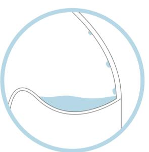
At the bottom of the dome is a full ring where the water is collected. The water then is funneled into a pipe and transported for immediate use. There is no salt in this new water, so it is very safe to drink.
