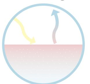
When water reaches a high enough temperature, the liquid is turned into a gas, and leaves any extra baggage behind (salt). The gas then rises to the top of the dome for the next phase in the process.
