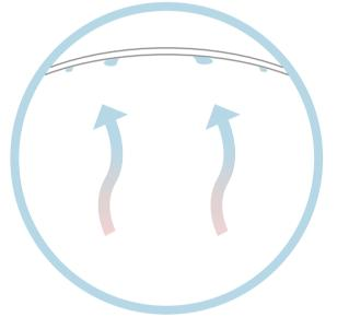
When the gas hits the top of the dome it cools back down to a pure, drinkable liquid. The water then travels the inner shell of the art piece and collects other droplets until it reaches the bottom.
